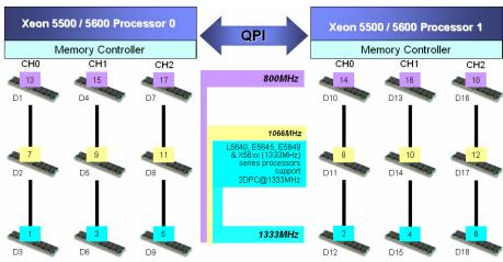
1-18: DIMM population sequence, D1-D18: DIMM slot assignments
